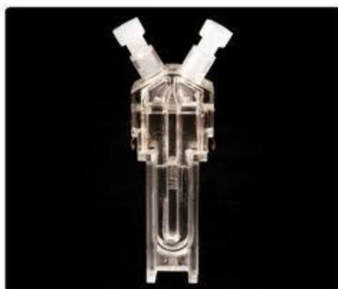
Figure 15 – Zetasizer Nano disposable capillary cell (DTS1070). This cell measures zeta potential and electrophoretic motility through electrodes. From www.malvernstore.com , accessed on 9 th April [72].
